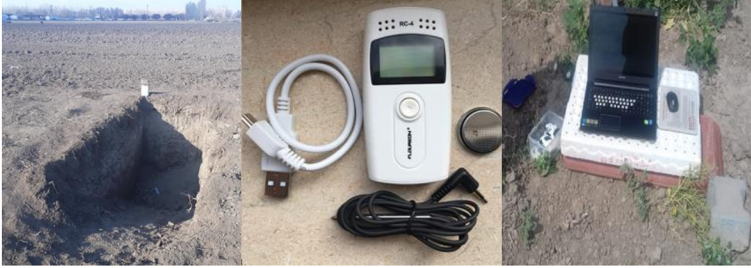
FIGURE 2. Placing the thermal sensors (Elitech RC-4 Mini temperature data logger) in soil profile
